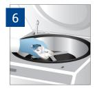
Place the BD SurePath Direct to Slide Kit Slide Holder with sample into a compatible centrifuge and spin at 200 g for 2 minutes.
