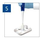
Slowly pipet 2 mL of sample into the BD Settling Chamber.
