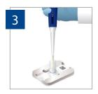
Pipet 1 mL of BD Density Reagent into the BD Settling Chamber.
