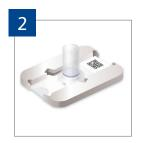
Place the labeled BD PreCoat™ Slide(s) into the BD SurePath™ Direct to Slide Kit Slide Holder. Attach a BD Settling Chamber.
